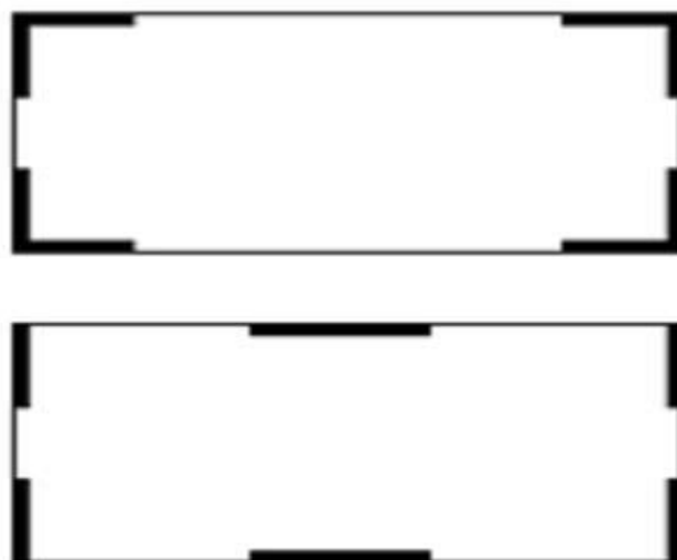
Figure 2.2 Effective Shear Wall Arrangement
