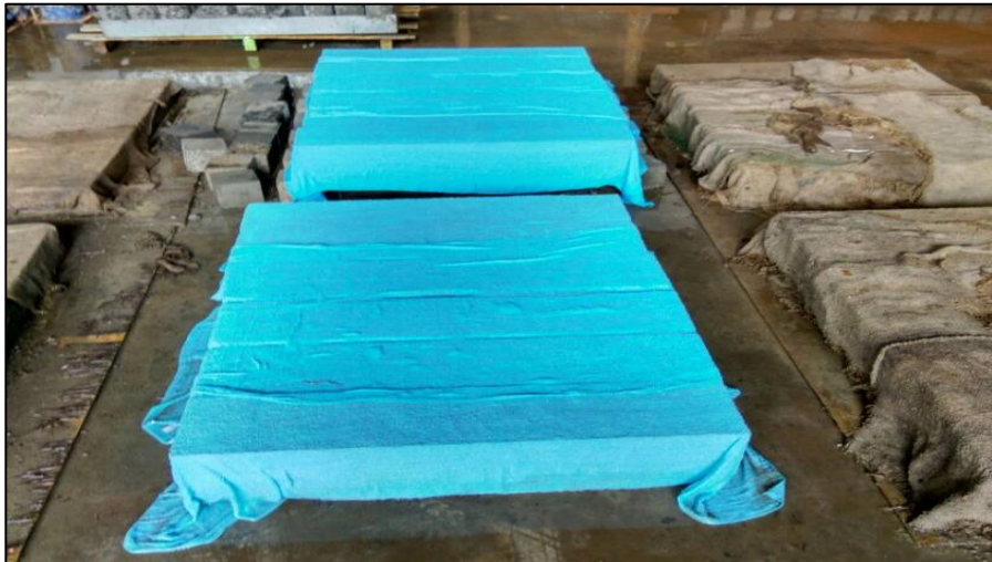
Figure 3.10: The Prism Coating by Gunny
