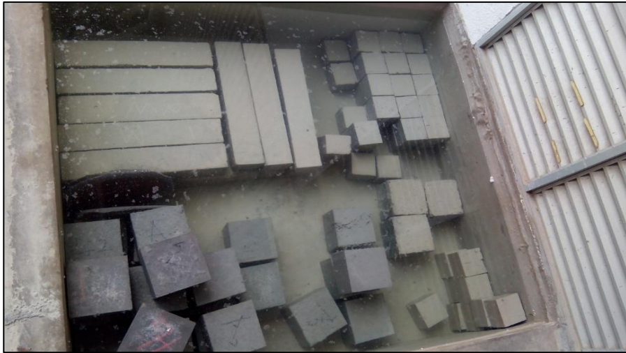
Figure 3.9: The Cube Concrete Immersed in Water Tank
