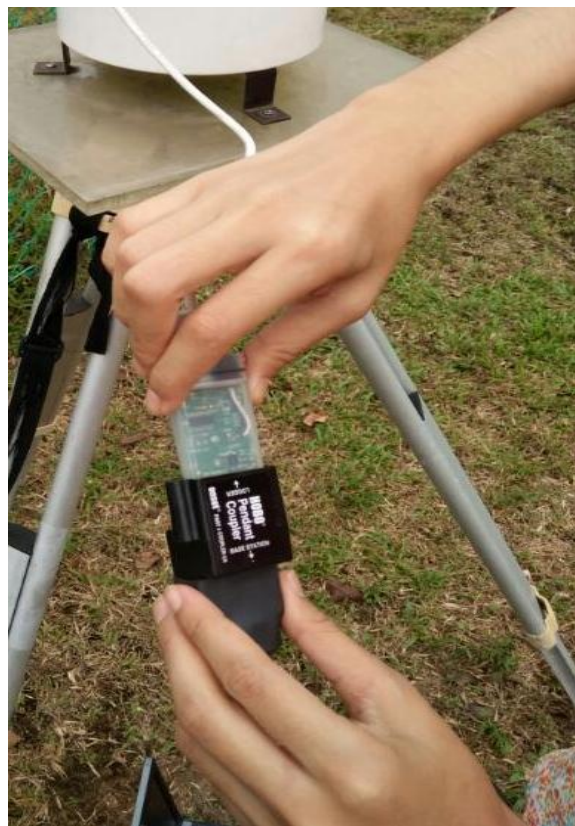
Figure 3.5.2 (b) Inserting logger into base station
