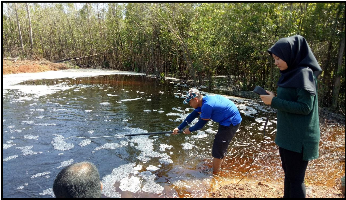
Figure 3.11.3 (c) Measuring velocities by using current meter
