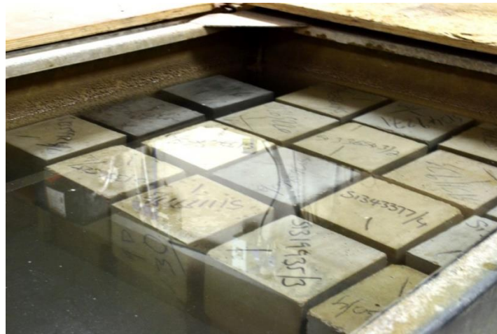
Figure 3.5 Full water curing for specimens
