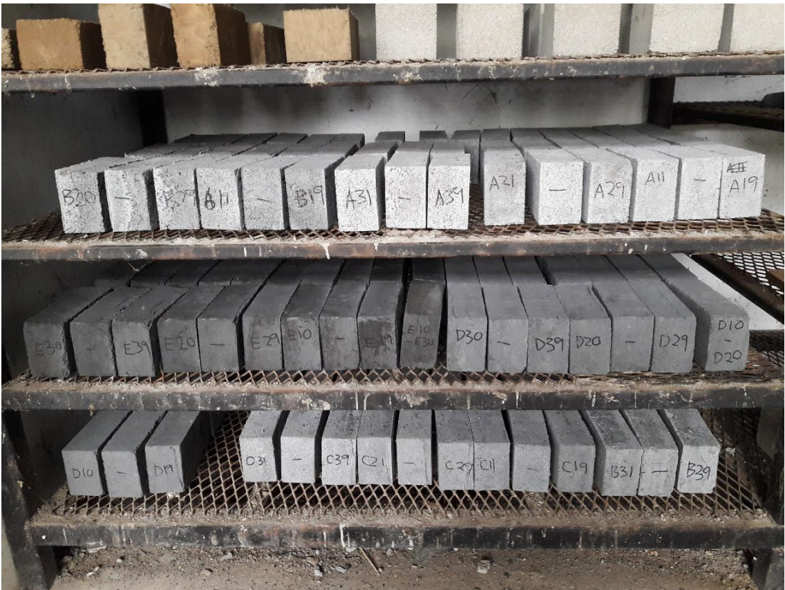
Figure 3.14 Brick was cured using air curing
