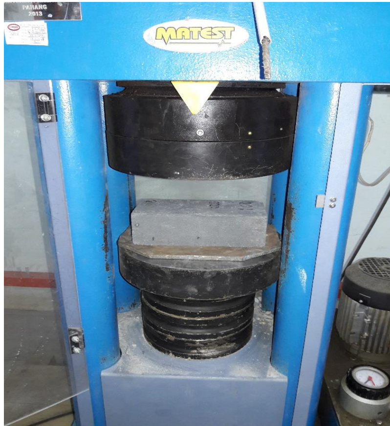
Figure 3.15 Brick under compressive strength test
