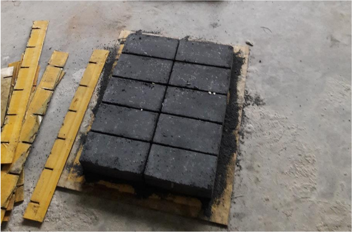
Figure 3.13 Unmould brick specimen
