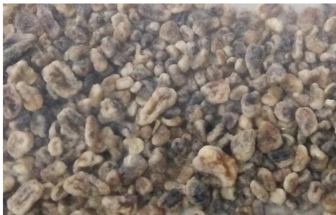
Figure 3.6 : Dried seaweed was blended to desired particle sizes, 0.7mm – 1.5mm.
