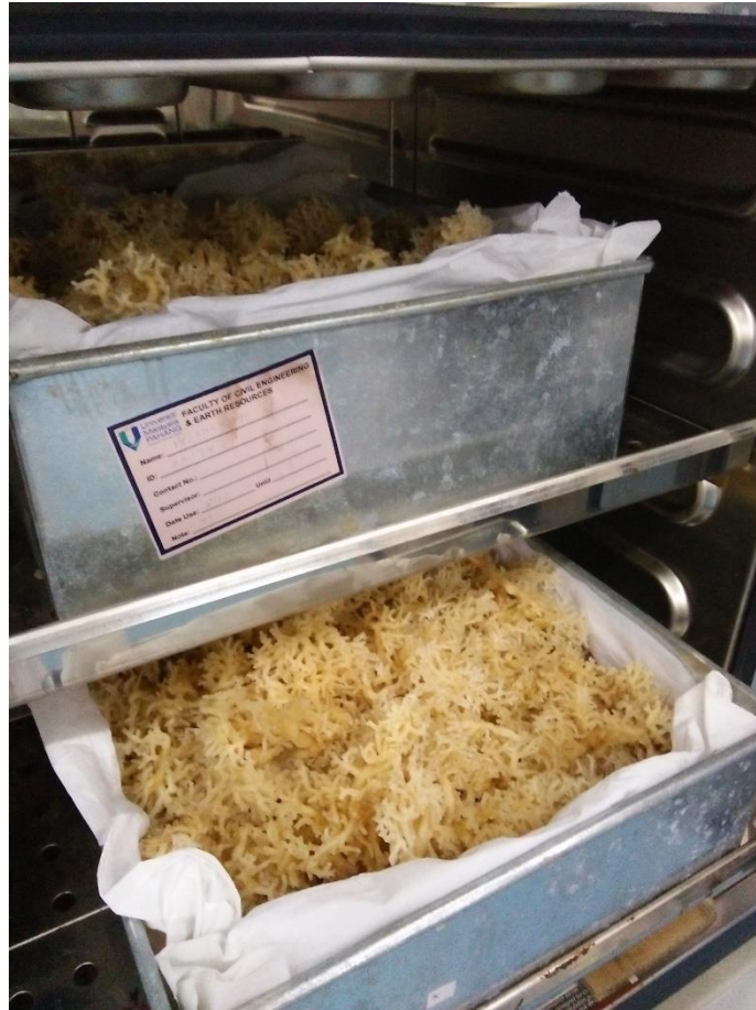
Figure 3.4 : Seaweed was oven-dried at 60°C for 24 hours
