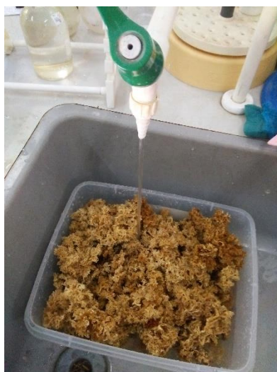
Figure 3.3 : Seaweed was first washed and rinsed with tap water, was thoroughly washed with doubly distilled water.
