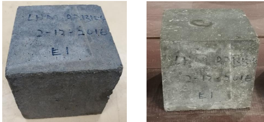
Figure 4.10 Physical Changes of Normal Concrete Before Immersion (left) and After Immersion in 5 % Sodium Chloride (right).
