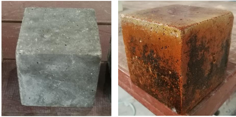
Figure 4.4 Physical Changes of Normal Concrete Before Immersion (left) and After Immersion in 5 % Hydrochloric Acid (right).
