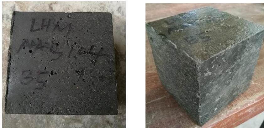
Figure 4.8 Physical Changes of SMCA Concrete Before Immersion (left) and After Immersion in 5 % Sodium Sulphate (right).
