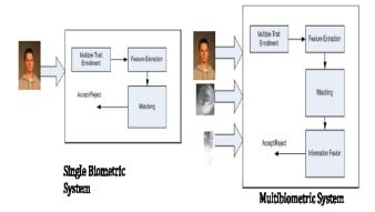
Fig. 3: Single Biometric vs. Multibiometric System
