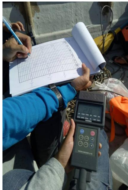
Figure 3.5 The Use of Conductivity Meter for Salinity Measurement
