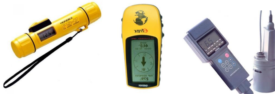
Figure 3.3 Equipment Used in Field Survey (from left: handheld depth sounder, GPS and water quality meter)
