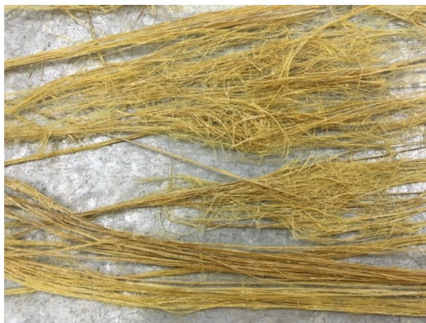
Figure 1. Macroscopic photograph of alkali treated bamboo fibers
