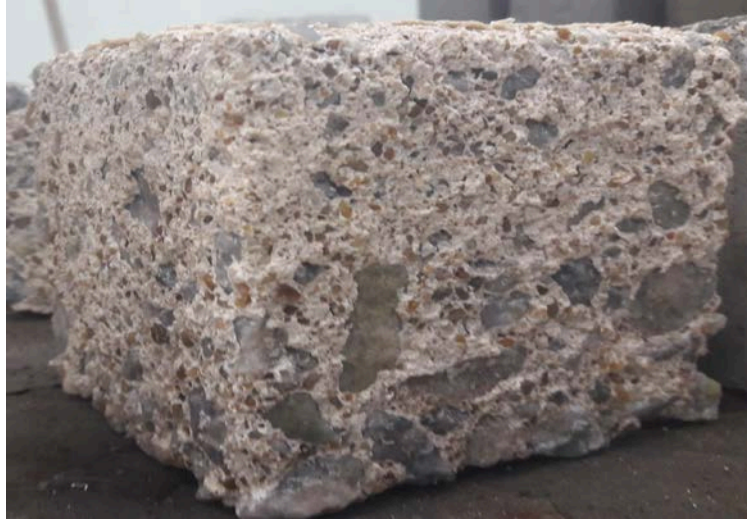
Fig 3 Eggshell concrete after submerged in sulphuric acid
