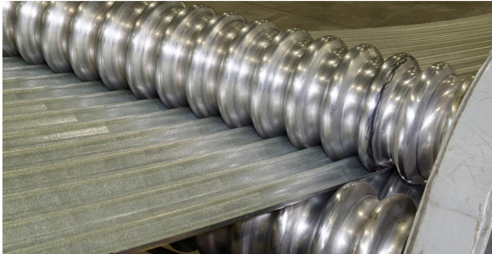
Figure 3.2 Roll forming process of cold-formed steel
