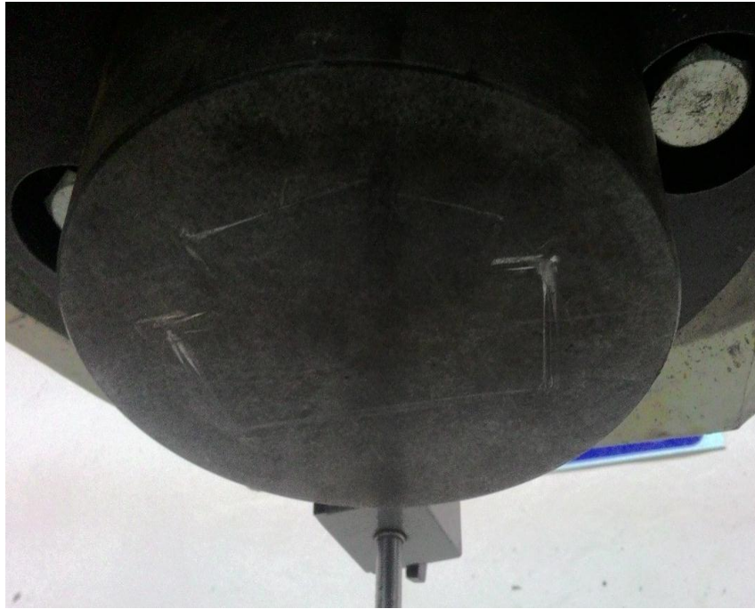
Figure 3.6 Bearing plate at the top
