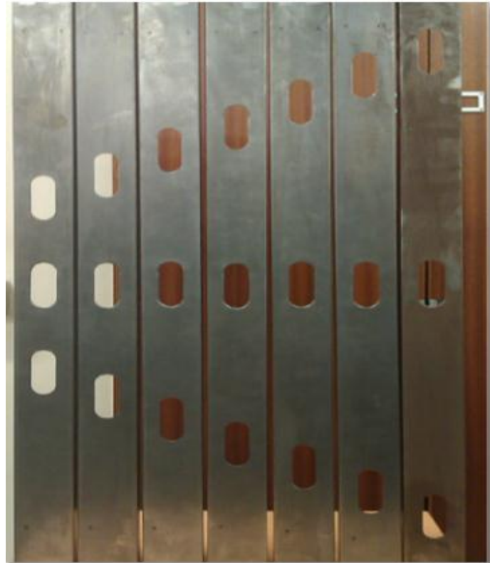
Figure 1.4 Example of cold-formed steel with different position of openings
