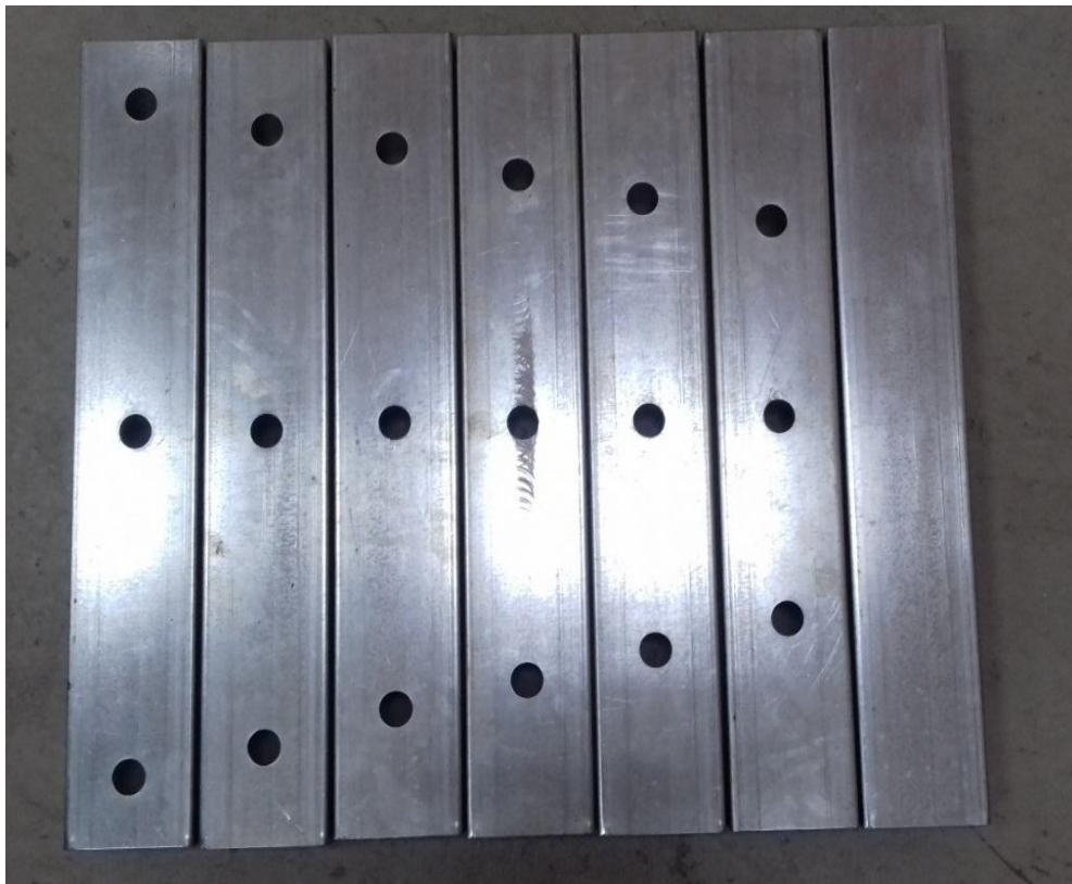
Figure 3.3 Series of cold-formed C section with various position of openings
