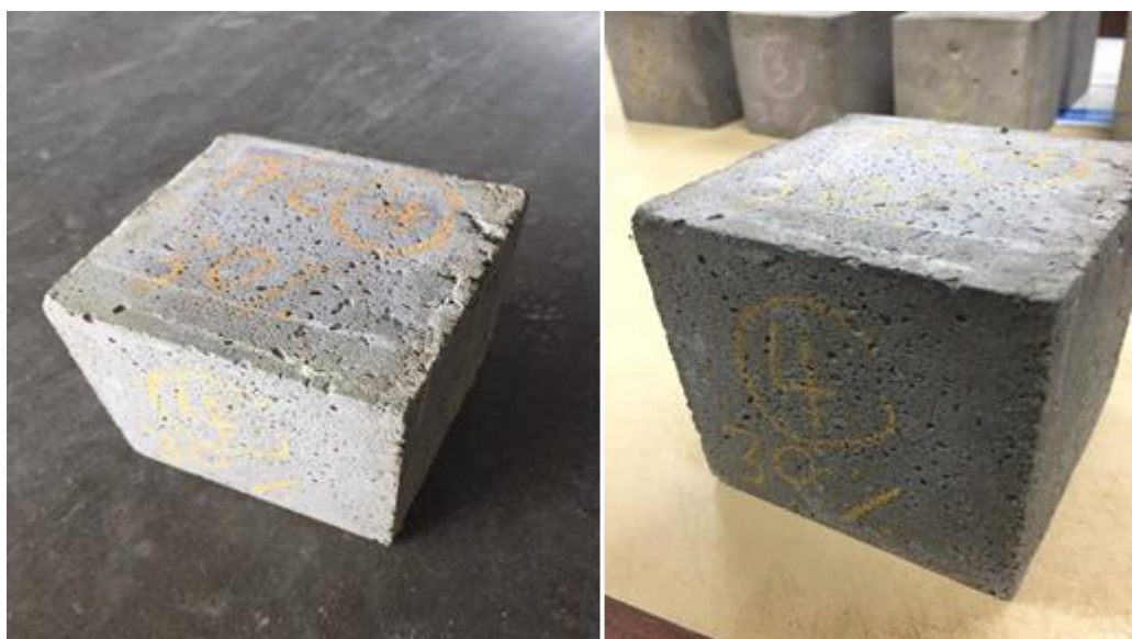
Figure 4.8 Deterioration before immersing in Sodium Chloride Solution and after 90days for Specimen with 30% PSBE
