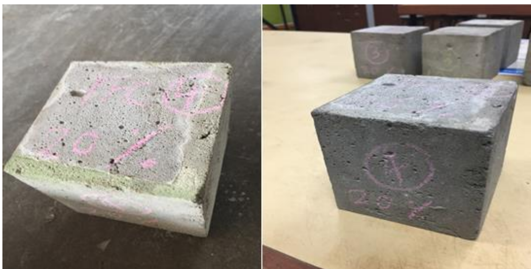
Figure 4.7 Deterioration before immersing in Sodium Chloride Solution and after 90days for Specimen with 20% PSBE
