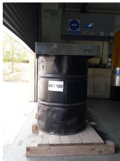
Figure 3.5: Conventional bitumen with grade 80 – 100
