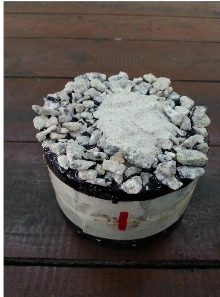
Figure 3.7: Asphalt concrete pavement sample undergoes volumetric patch method
