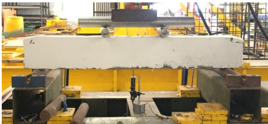
Figure 3.13 Flexural strength test
