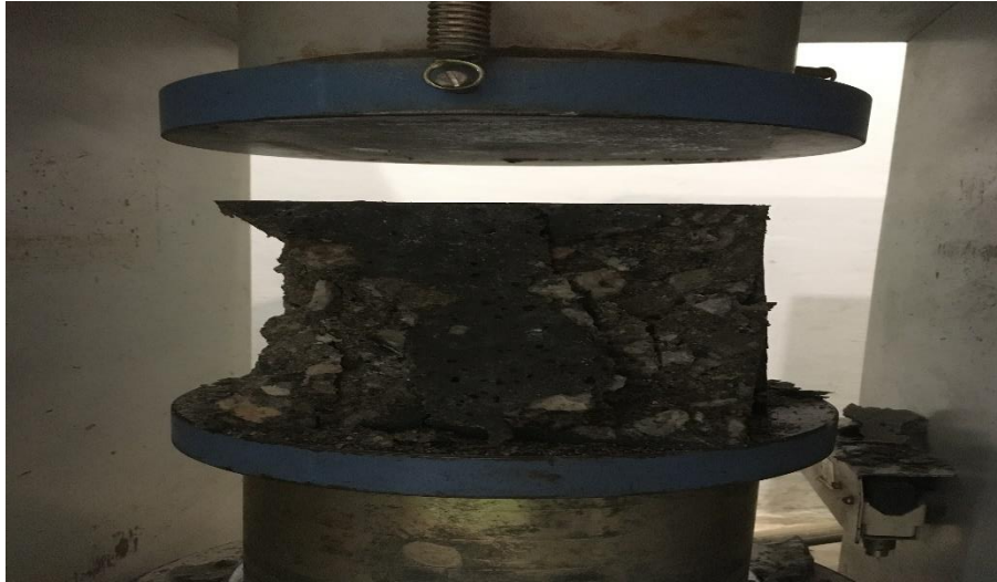
Figure 3.12 Compressive Strength test
