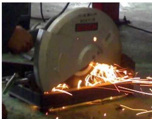
Figure 3.16: Cutting angle on steel bar
