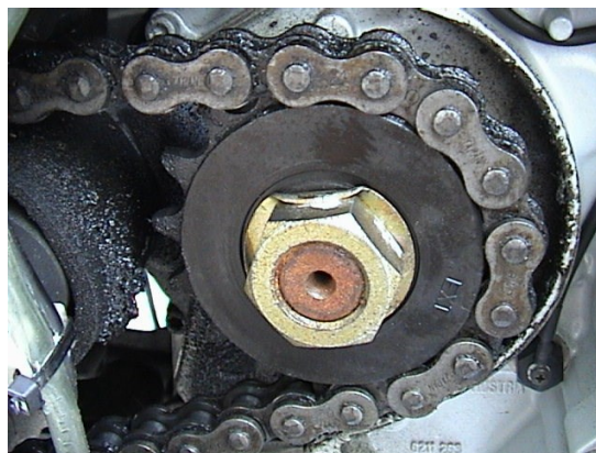
Figure 2.13: Chain and sprocket joining
