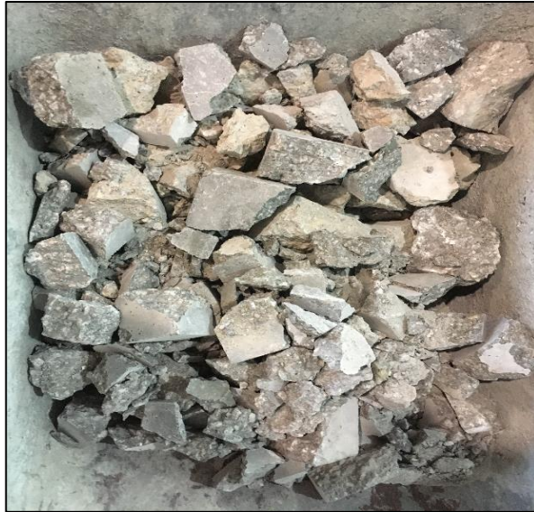
Figure 3-7: RCA after crushing process
