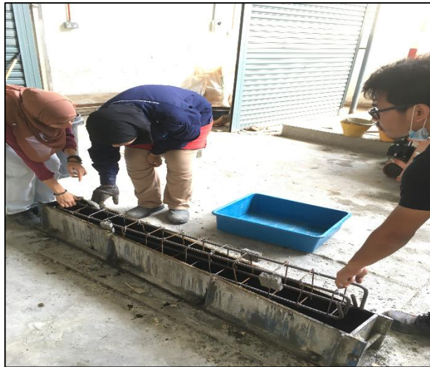
Figure 3-12: Installation of rebar
