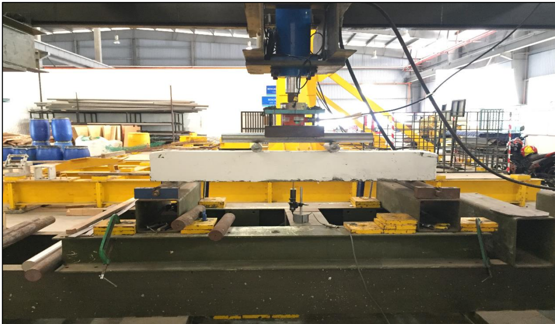
Figure 3-22: Flexural Test setup
