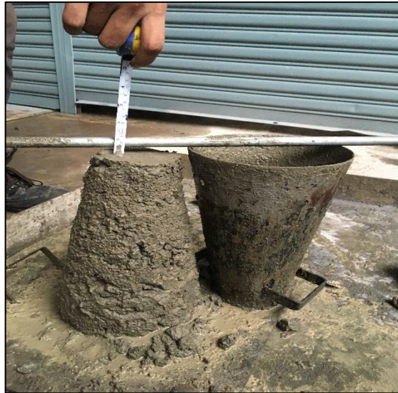
Figure 3-19: Concrete Slump Test Results
