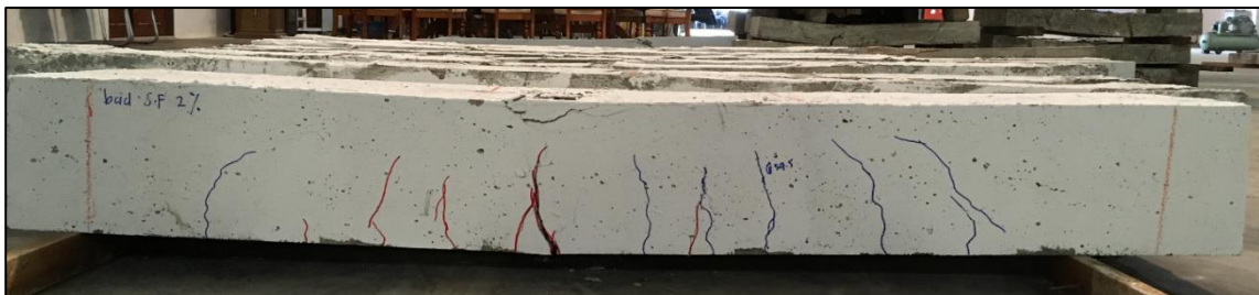
Figure 4-16: Cracking Pattern of RCA-SF2% beam
