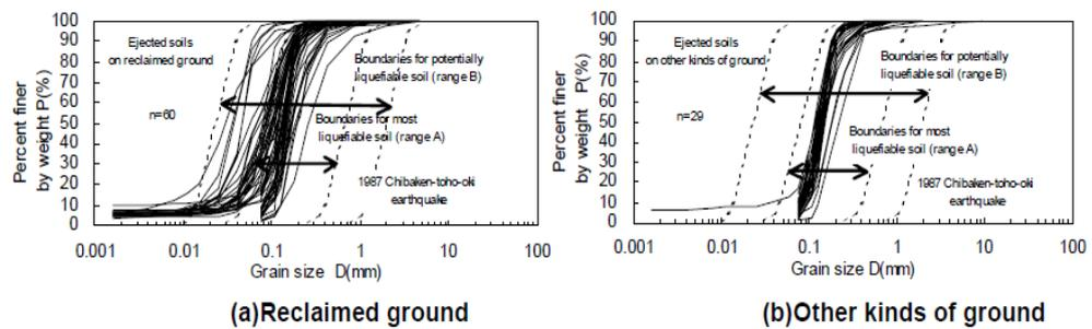
Figure 2.4 Comparison of soil samples using the Technical Standards of Ports and Harbor
