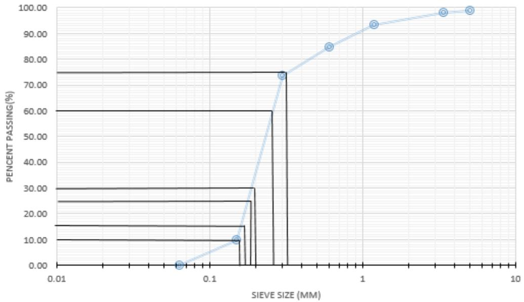
Figure B3: Determination of  $D_{10}$ ,  $D_{15}$ ,  $D_{30}$ ,  $D_{60}$  of Pantai Bati Hitam before crushing
