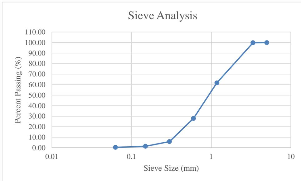
Figure A6: Particle size distribution of Teluk Cempedak soil sample after crushing
