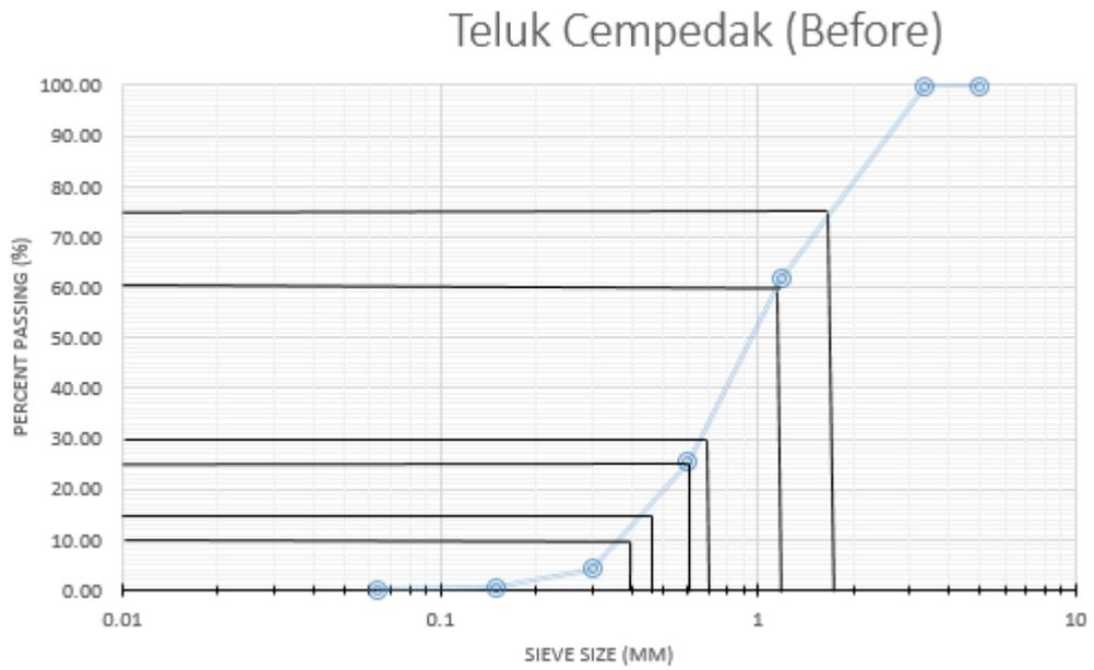
Figure B5: Determination of  $D_{10}$ ,  $D_{15}$ ,  $D_{30}$ ,  $D_{60}$  of Teluk Cempedak before crushing
