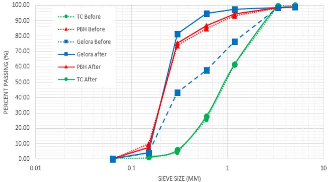
Figure 4.1: Particle Size Distribution of soil samples.
