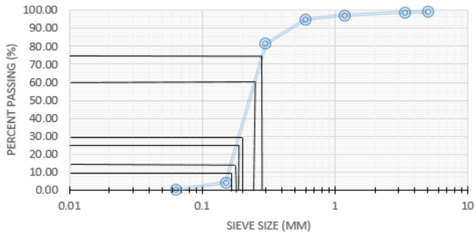
Figure B2: Determination of  $D_{10}$ ,  $D_{15}$ ,  $D_{30}$ ,  $D_{60}$  of Taman Gelora after crushing
