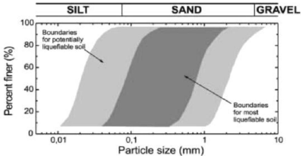
Figure 2.1 Liquefaction Potential based on Particle Size Distribution
