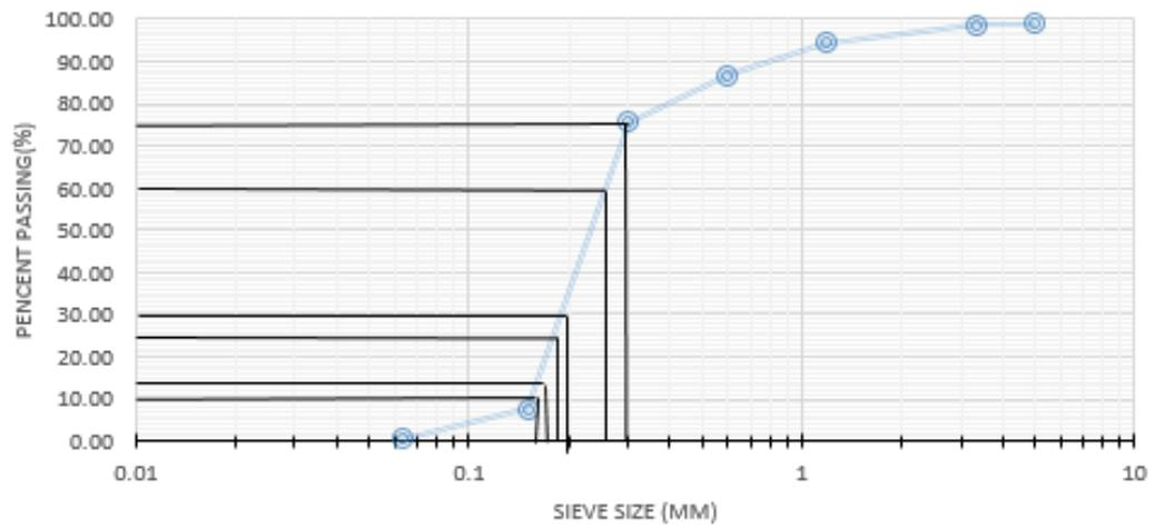
Figure B4: Determination of  $D_{10}$ ,  $D_{15}$ ,  $D_{30}$ ,  $D_{60}$  of Pantai Batu Hitam after crushing
