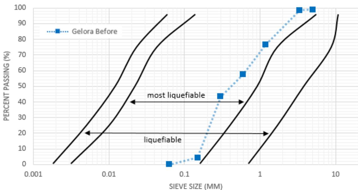
Figure 4.3: Comparison with Technical Standard of Ports and Harbour of Japan of soil samples ( $U_c \geq 3.5$ )
