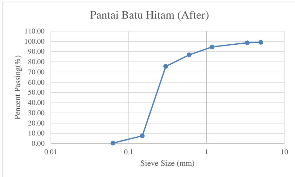
Figure A5: Particle size distribution curve of Pantai Batu Hitam after crushing
