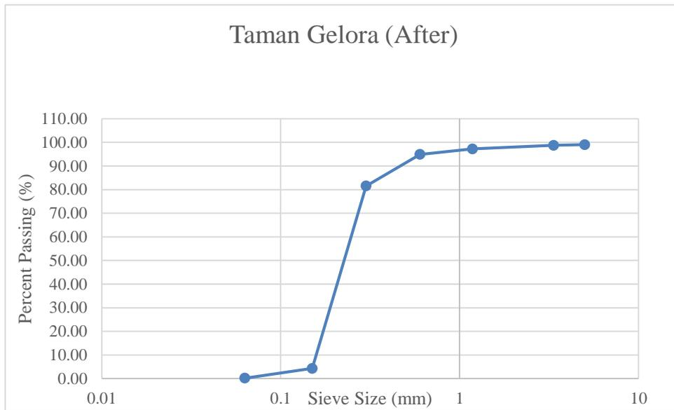
**Figure A4:** Particle size distribution curve of Taman Gelora soil sample after crushing
