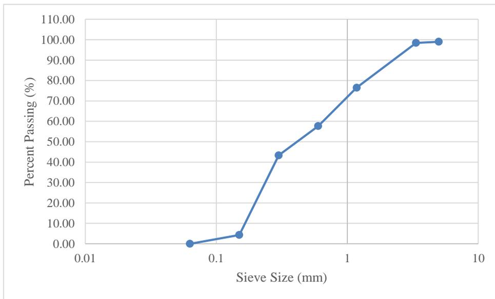
**Figure A1:** Particle size distribution curve of Taman Gelora soil sample before crushing
