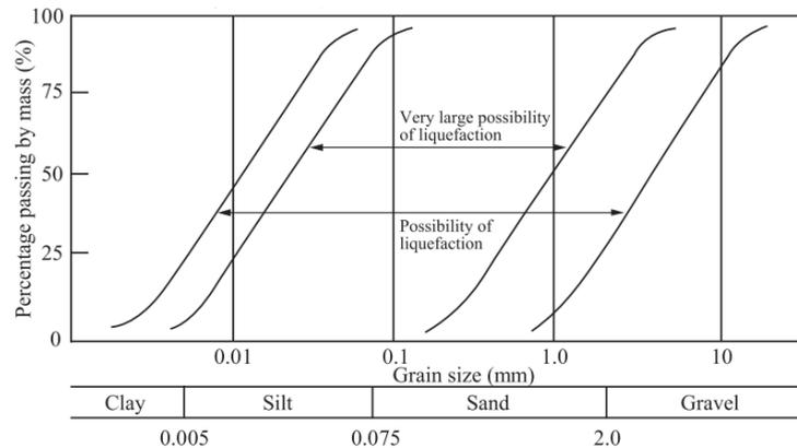
Figure 2.2 Possibility of Liquefaction with Large Uniformity Coefficient ( $U_c \geq 3.5$ )
