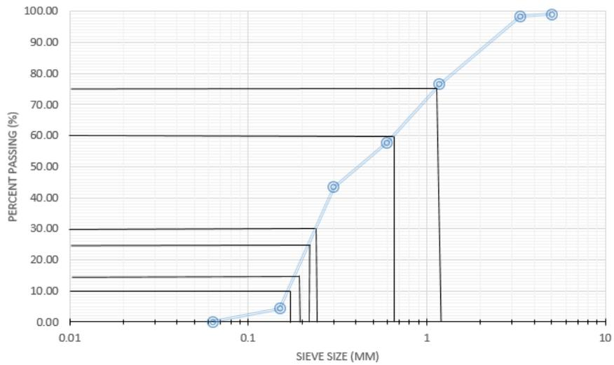
Figure B1: Determination of  $D_{10}$ ,  $D_{15}$ ,  $D_{30}$ ,  $D_{60}$  of Taman Gelora before crushing
