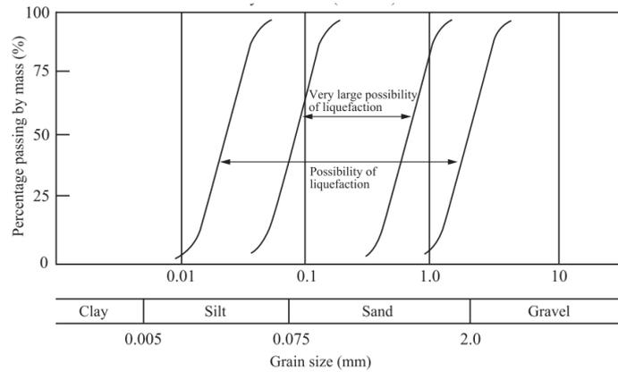
Figure 2.3 Possibility of Liquefaction with Small Uniformity Coefficient ( $U_c \leq 3.5$ )
