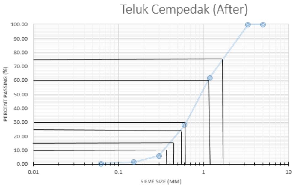
Figure B6: Determination of  $D_{10}$ ,  $D_{15}$ ,  $D_{30}$ ,  $D_{60}$  of Teluk Cempedak after crushing
