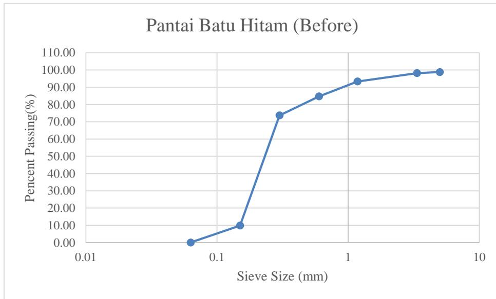
Figure A2: Particle size distribution curve of Pantai Batu Hitam soil sample before crushing
