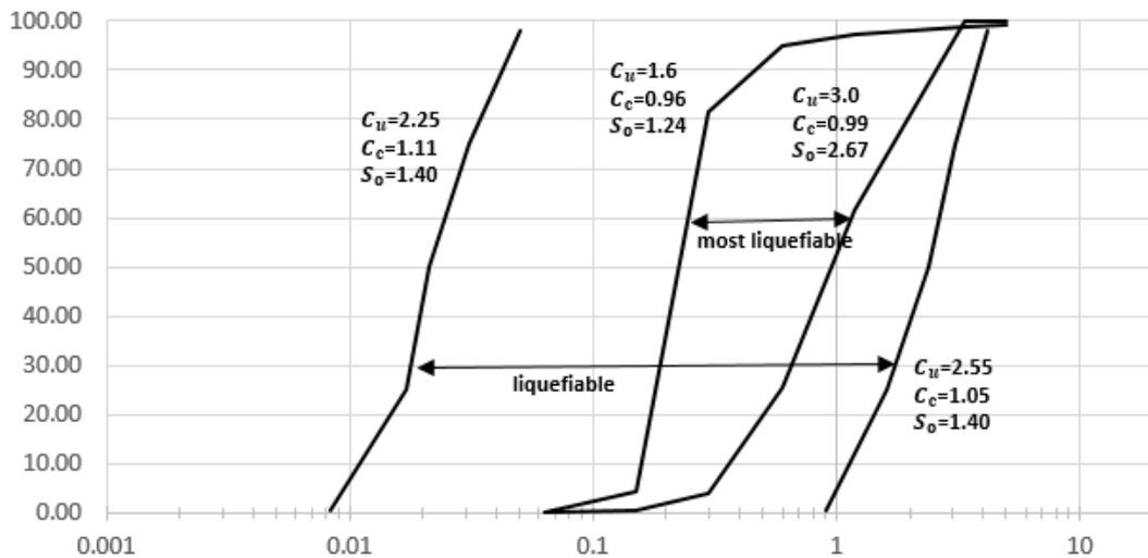
Figure 5.1: Guideline for Liquefaction potential for Kuantan coastal area
