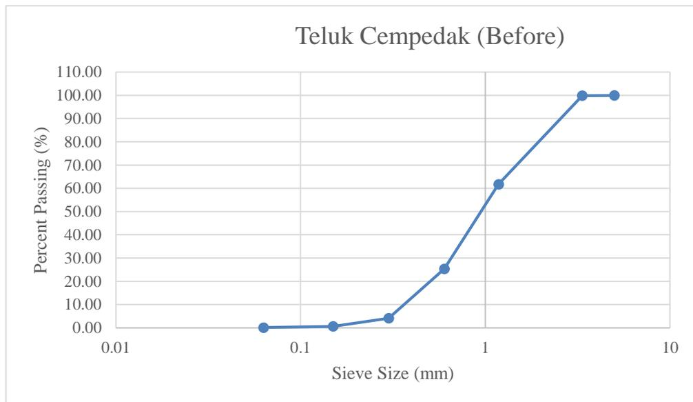
Figure A3: Particle size distribution curve of Teluk Cempedak soil sample before crushing
