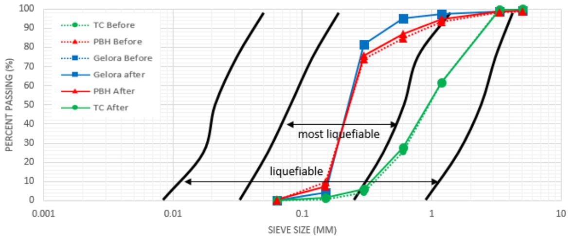
Figure 4.2: Comparison with Technical Standard of Ports and Harbour of Japan of soil samples ( $U_c \leq 3.5$ )
