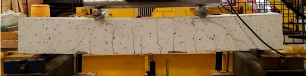
Figure 4.14 : Cracking pattern for 25% of RCA with 2% of Steel fibre( RCA2)
