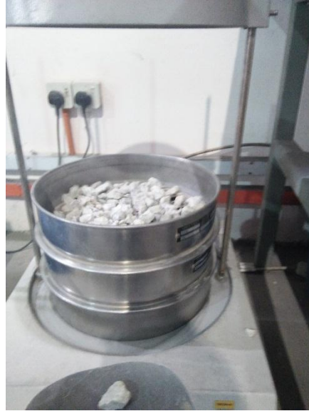
Figure 3.2: Sieve recycle concrete aggregate into 15mm -20mm
