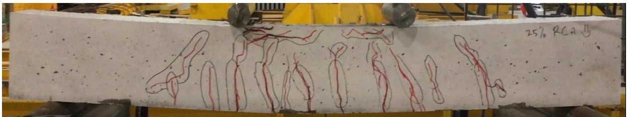
Figure 4.12 : Cracking pattern for 25% of RCA(RCA)
