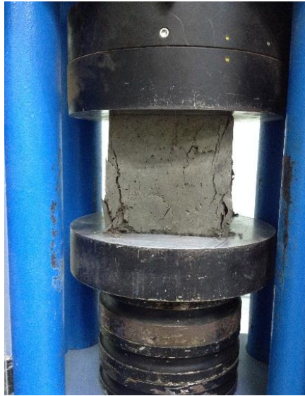
Figure 3.4: Compressive Strength Test
