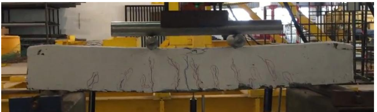
Figure 4.13 : Cracking pattern for 25% of RCA with 1% of Steel fibre(RCA1)
