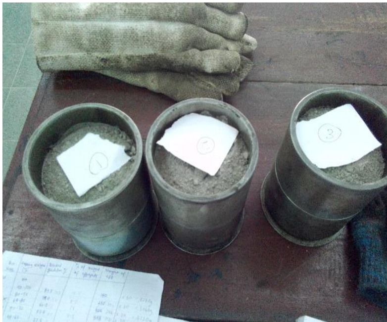
Figure 3-1 Mould with 101.6mm and 76.6mm high
