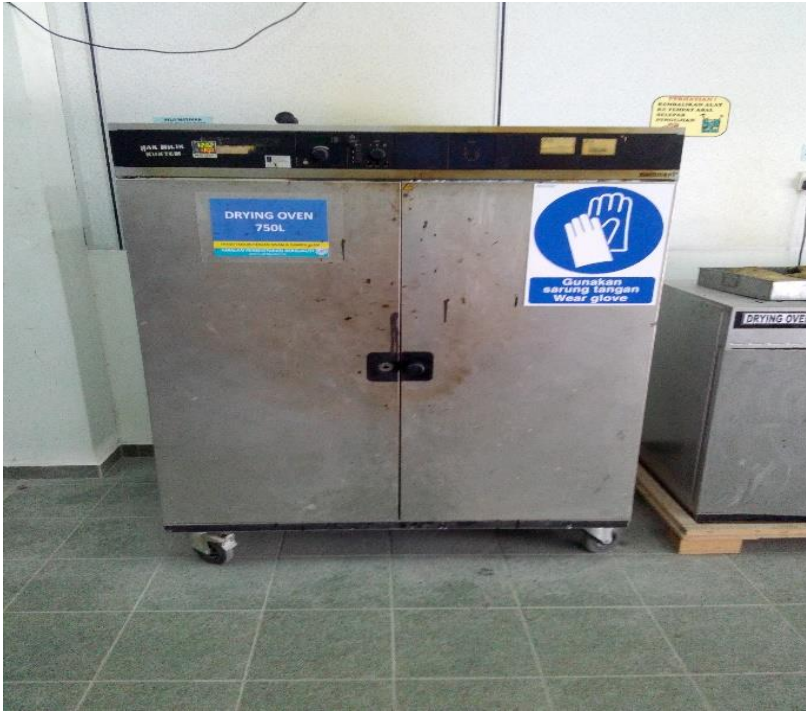
Figure 3-2 Drying oven ( 140 – 170° C)
