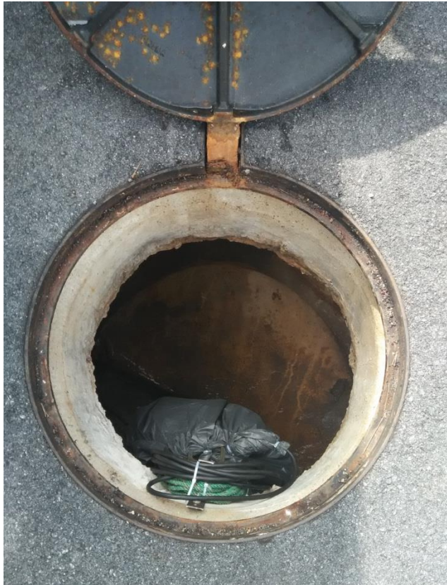
Figure 3.7 Set up of flow meter in the manhole
