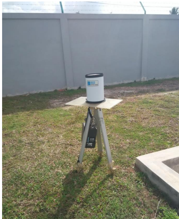
Figure 3.8 Set up of rain gauge in the open field
