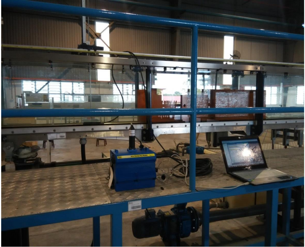
Figure 3.6 Calibration of flow meter
