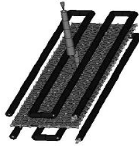
Figure 2.3: Cooling system design in Moldflow software
