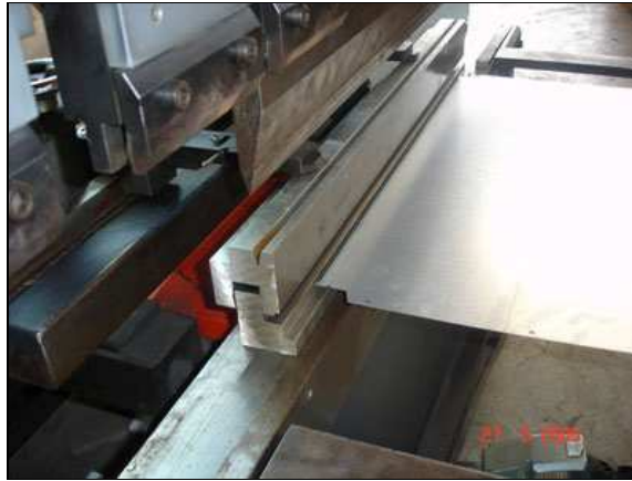
Figure 3.12: Process of bending sheet metal
