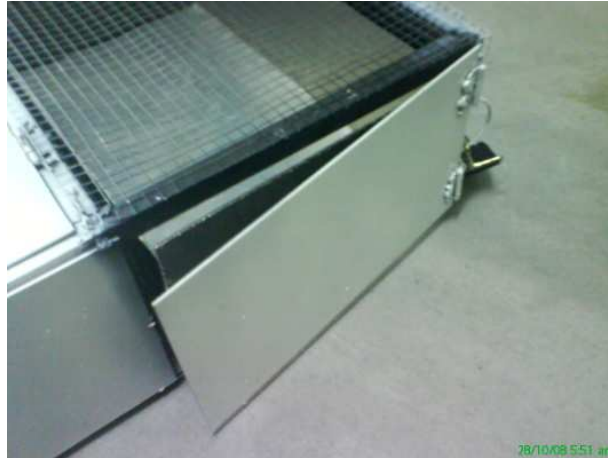
Figure 4.7: Door cannot be closed properly
