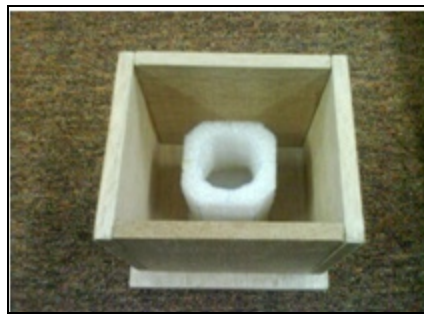
Figure 3.9: Place the master pattern in a box
