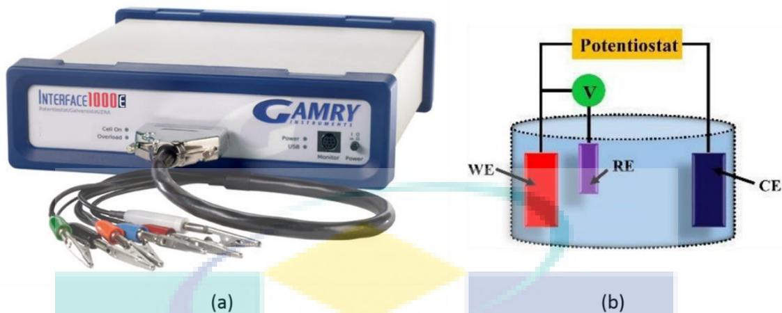
Figure 3.3 (a) Photograph of potentiostat used in this research (b) principle of three electrode measurement.
