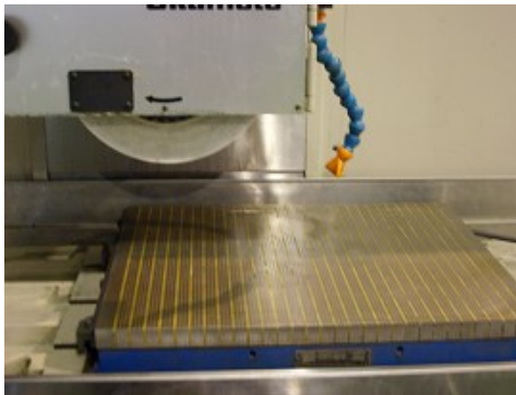
Figure 3.4: The working table, wheel head and coolant hose.
