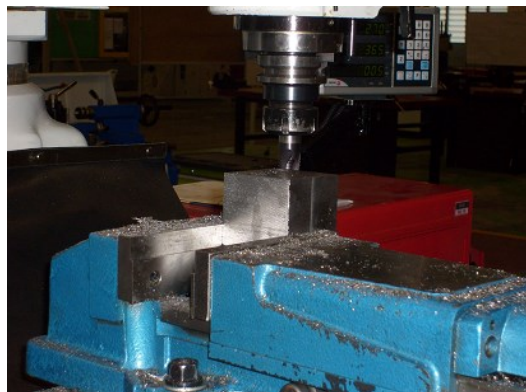
Figure 3.13: The milling machine to make the T- shape
