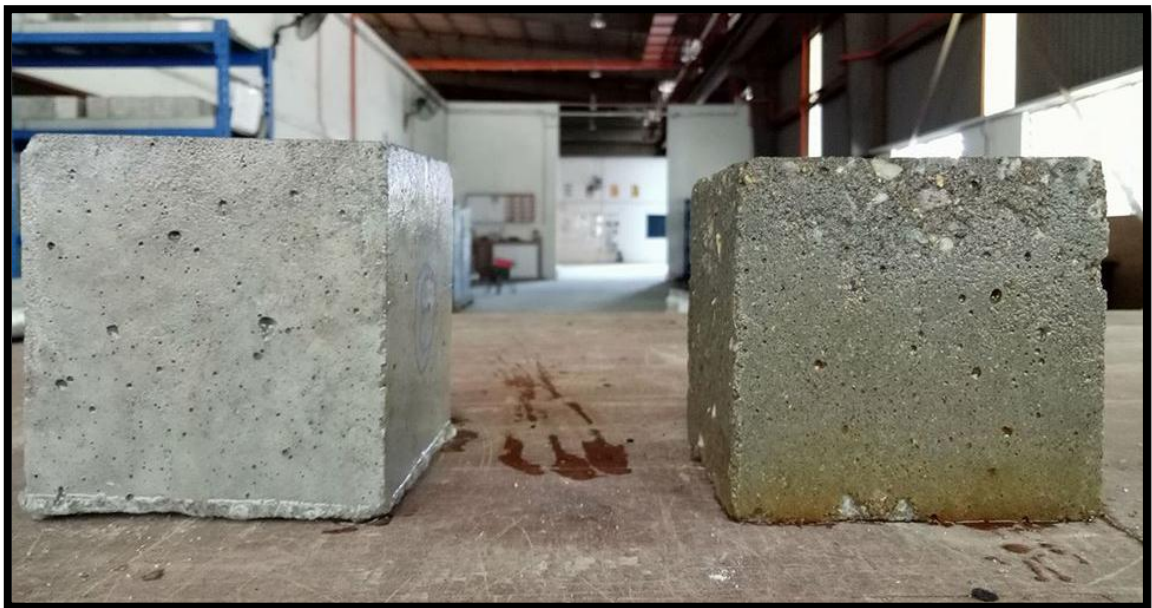
Figure 4.12 The comparison of specimen that contains 5% POFA before and after immersing in acid solution
