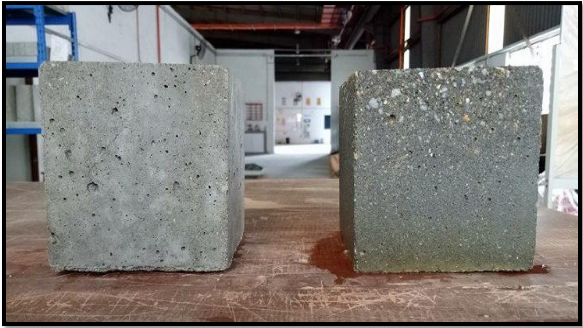
Figure 4.15 The comparison of specimen that contains 20% POFA before and after immersing in acid solution
