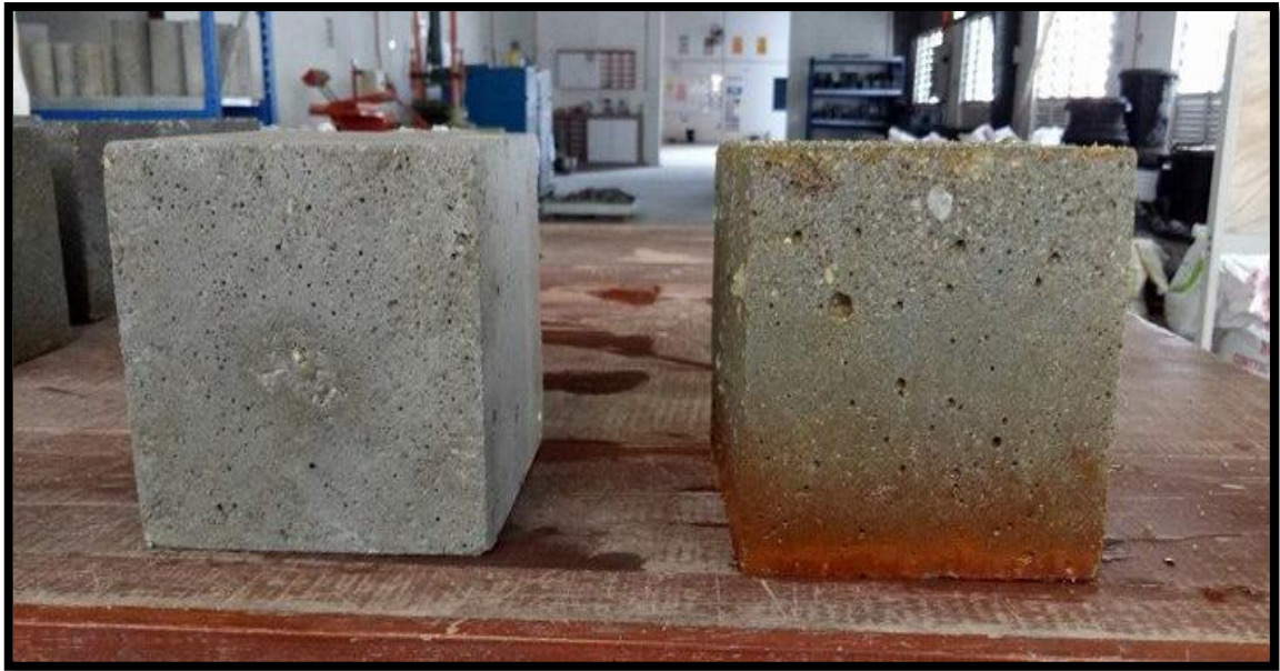
Figure 4.11 The comparison of control specimen before and after immersing in acid solution
