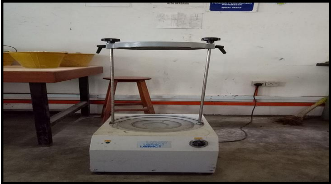
Figure 3.5 Sieving machine was used to sieve POFA
