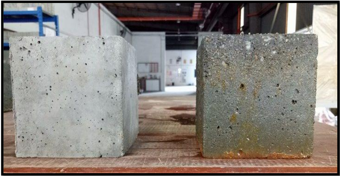
Figure 4.13 The comparison of specimen that contains 10% POFA before and after immersing in acid solution
