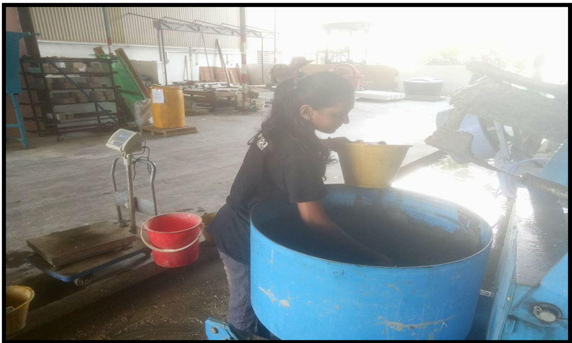
Figure 3.10 Casting of concrete specimen
