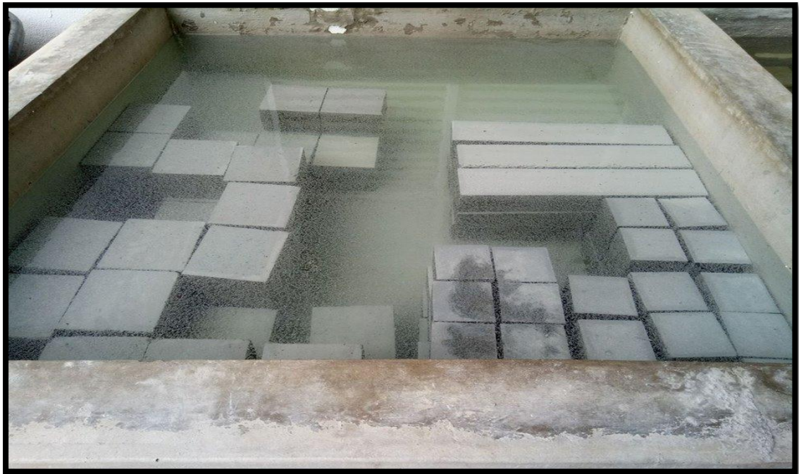
Figure 3.11 The concrete cubes were cured in the water tank
