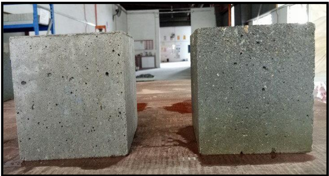
Figure 4.14 The comparison of specimen that contains 15% POFA before and after immersing in acid solution
