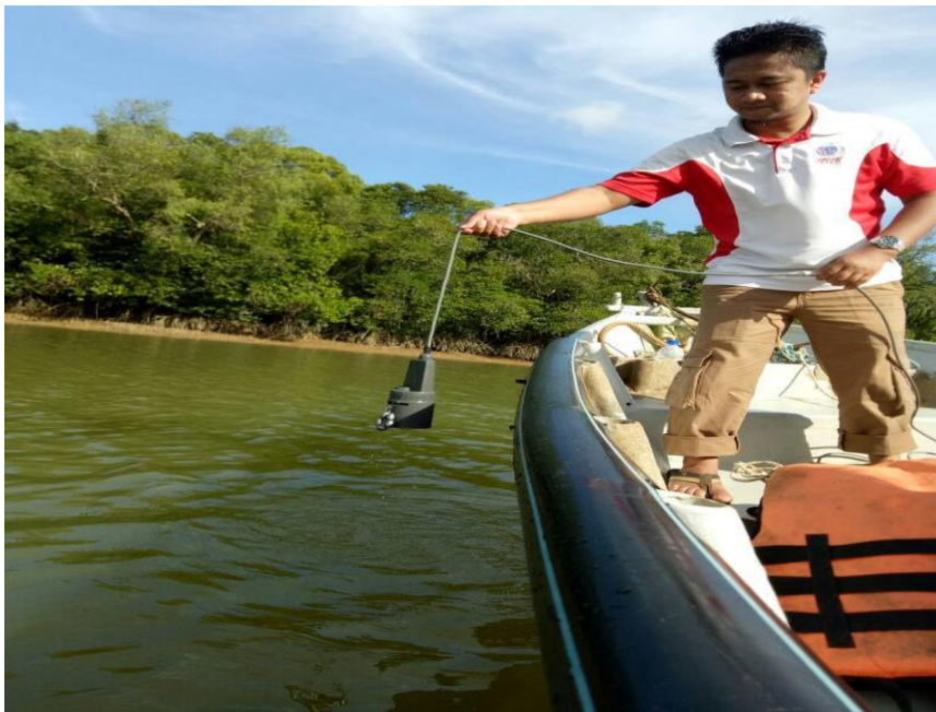
Figure 3.8 Horiba Water Quality Meter is used to record salinity readings for every one-meter vertical from the bottom to the water surface
