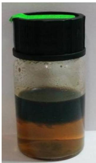
**Figure 4.1:** Distillate product of RSO by using FCC
