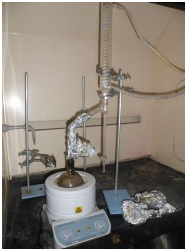
Figure 3.2.4 Experimental Setup (Dean Stark apparatus)
