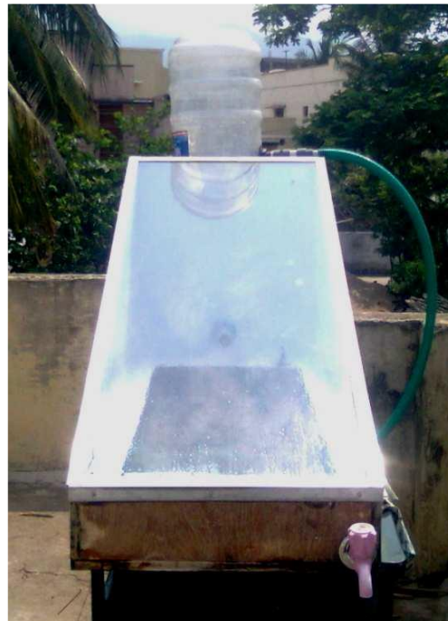
Figure 2-6: Solar Still with Copper Coating (Gnanadason, et al., 2011)
