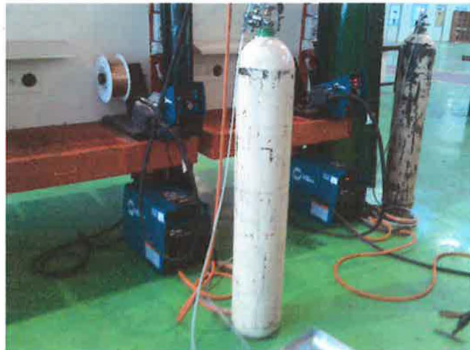
Metal inert gas welding
