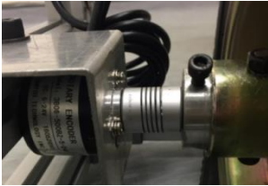
Fig.4: The position of encoder and wheels
