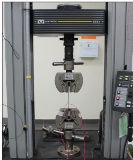
Fig.4. Tensile test using INSTRON 5567 Universal Testing Machine
