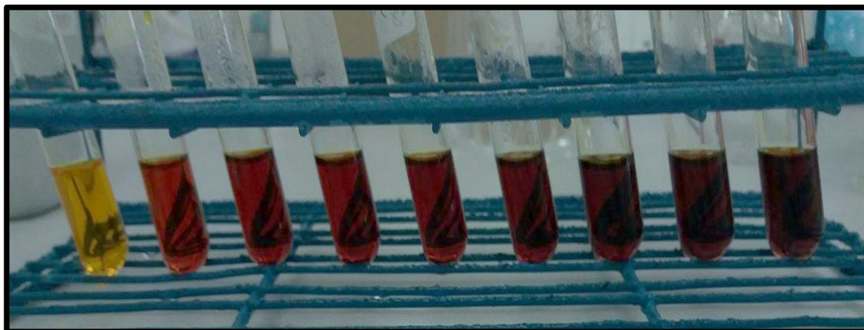
**Figure 4.7** : Standard xylose solution with DNS assay after the heating process
