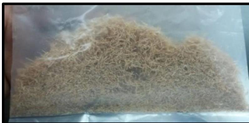
**Figure 3.1: Fresh oil palm frond fibre**
