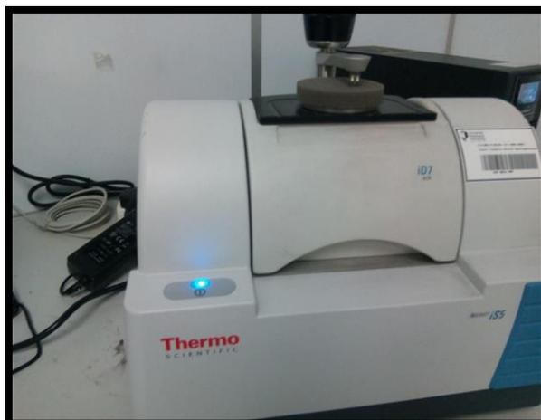
**Figure 3.7** : Fourier transform infra-red spectrometry
