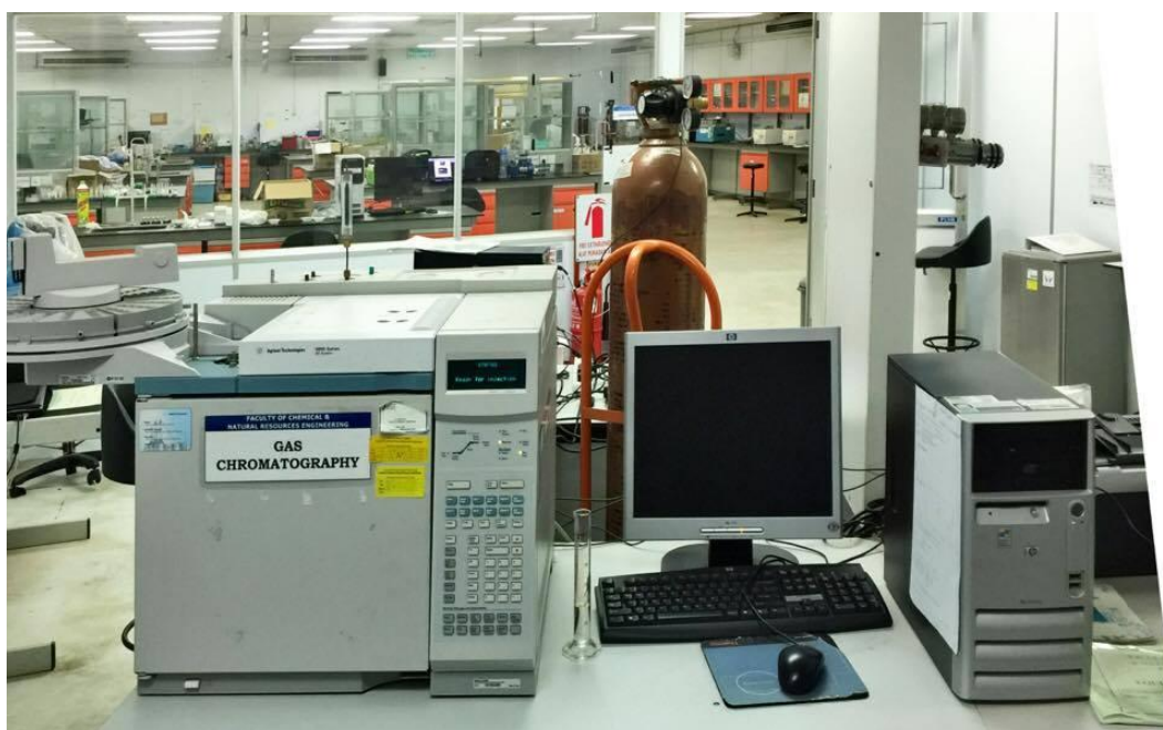
Figure 3.4: Gas chromatograph 6890 Series that was used to detect the permanent gases (CH 4 , CO 2 and CO)
