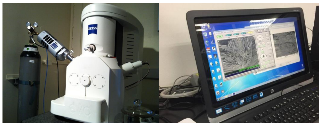
Figure 3.7: Scanning Electron Microscopy (SEM) EVO-50 that was used to take SEM images
