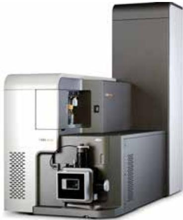
*Liquid Chromatography QTOF Mass Spectrometer (LCQTOF/MS) Vion IMS (Unifi 1.8), Waters, UK*
