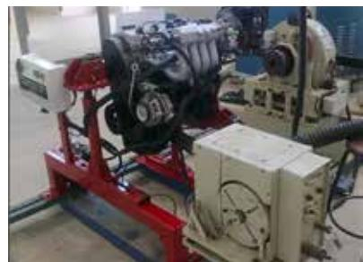
Eddy Current Dynamometer (100KW)
