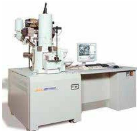
*Field Emission Scanning Electron Microscope*
