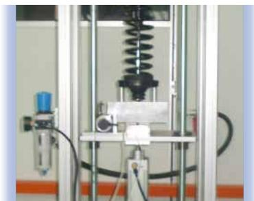
Shock Absorber Test Rig
