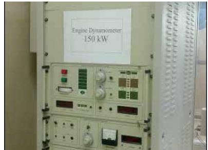
Dynamometer Control Panel
