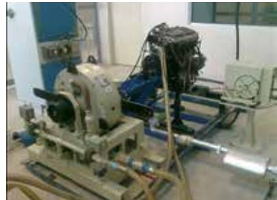
Eddy Current Dynamometer (150KW)
