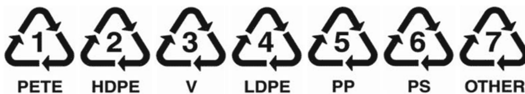
Figure 1.1: Marks of the seven types of plastics on various plastic products (The Society of the Plastic Industry [SPI], 1999)
