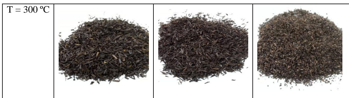
Figure 4-1: The raw biomass particles and their torrefied products at different torrefaction temperatures for 30 minutes.
