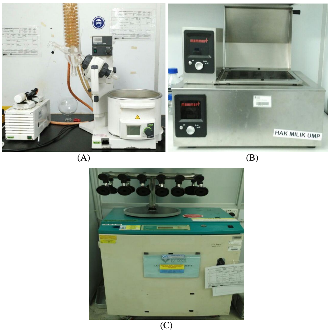
Figure 3.2: Photograph of equipment. (A) Rotary vacuum evaporator (B) Water bath shaker (C) Freeze dryer
