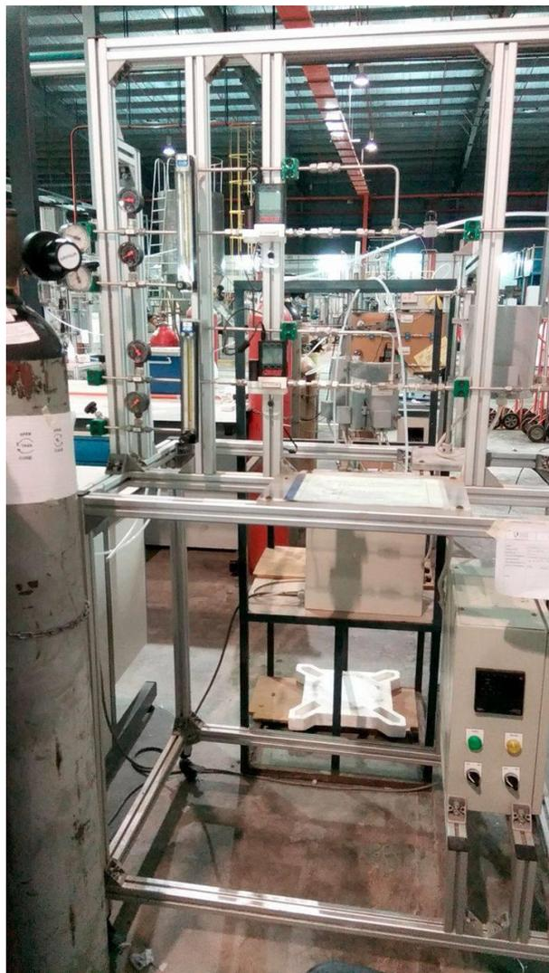
Figure A-1: Gas catalytic reactor.
