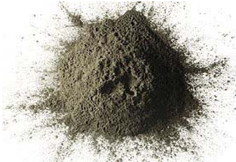
Figure 2.2: Palm oil mill fuel ash waste (POMFAW)
