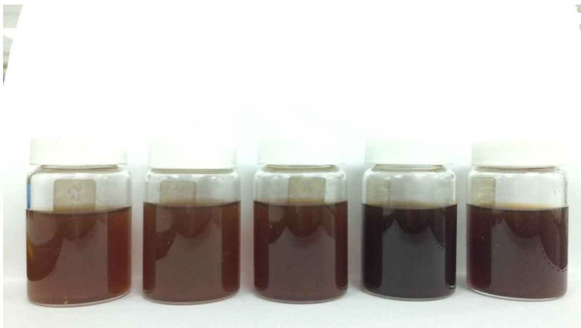
The extract samples at different solid to solvent ratio.
