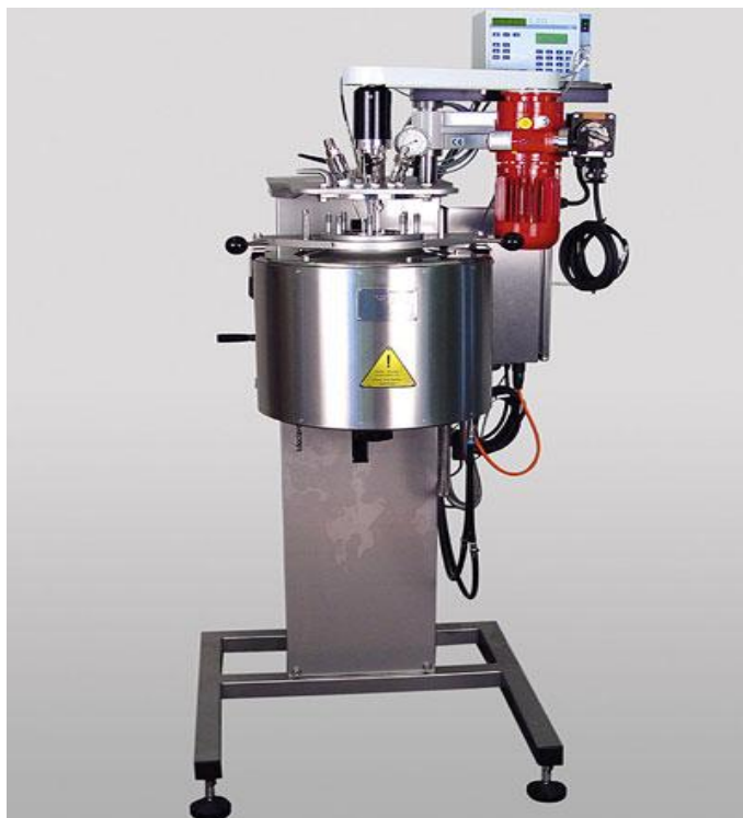
Kiloclave Laboratory Pressure was used as SWE
