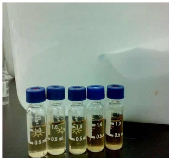
Sample in the vial was prepared for HPLC analysis
