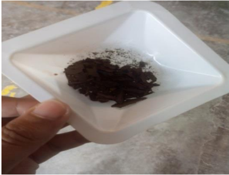
Picture 1: Weight of corrodes or deposited inside the solution = 7.021 g
