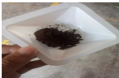
Picture 2: Weight of corrodes or deposited inside the solution = 10.883g
