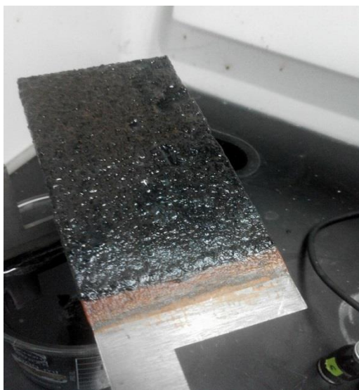
Black deposited of FeS on the anode electrode after EC treatment
