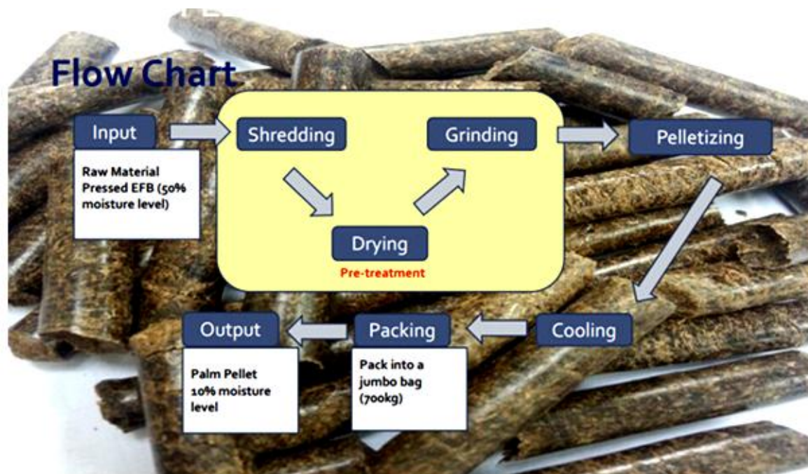
Figure 2-6 : OPT Pellet Production procedure( Huang ,2014 )
