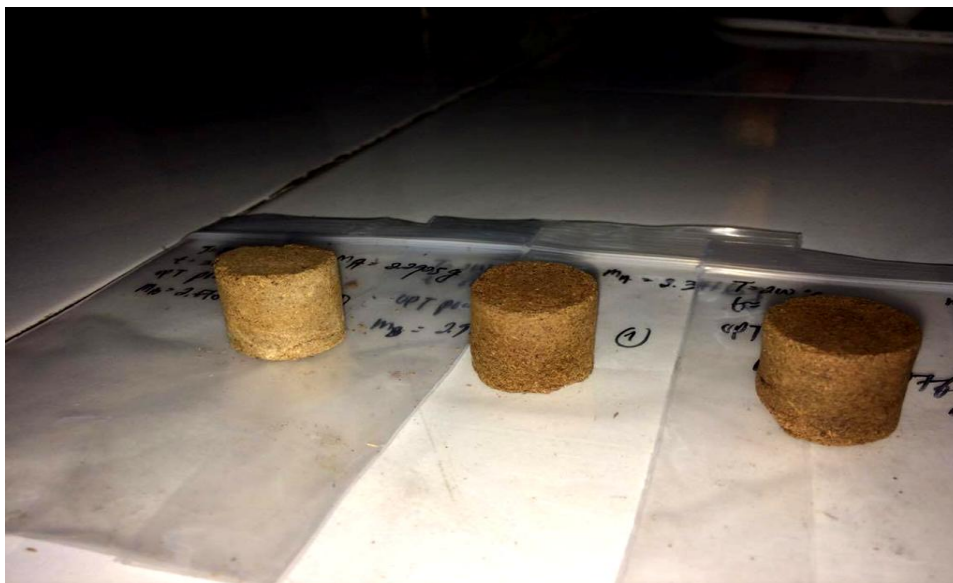
Figure 4-4 : Colour change of OPT powder pellet towards three different torrefaction temperatures at 30 minutes
