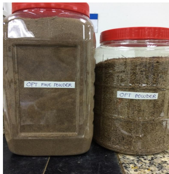
Figure 3-3 : OPT fine powder and fiber as raw material
