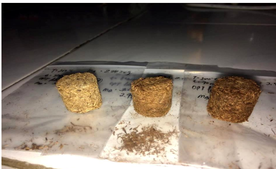
Figure 4-5: Colour change of OPT fiber pellet towards three different torrefaction temperatures at 30 minutes
