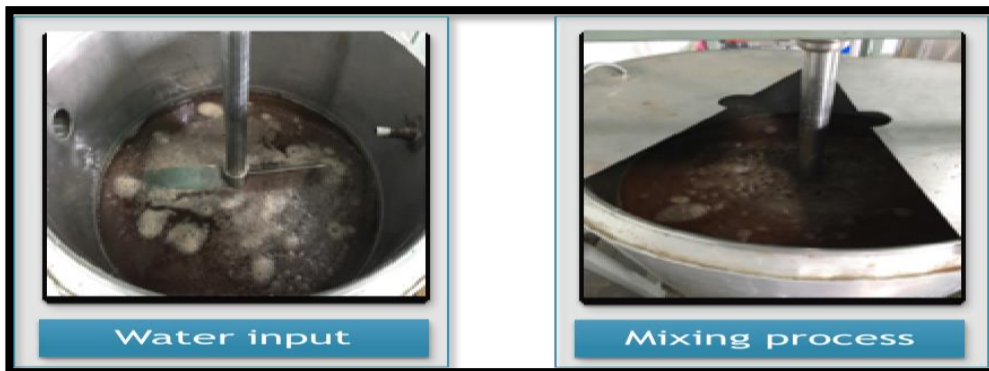
Figure 3.2: Water inlet and mixing- reaction in delignification process
