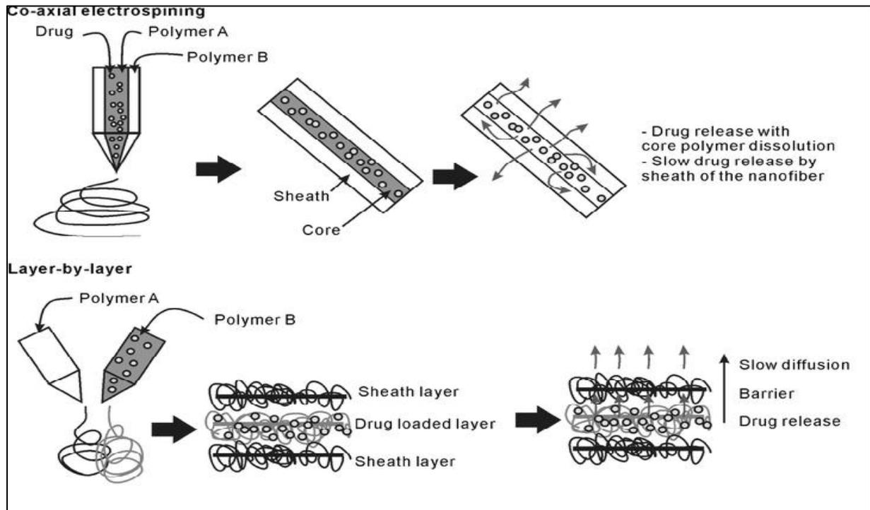
**Figure 0.4:** Schematic diagram of drug loaded nanofiber with sheath layer and its drug release kinetics (Son et al., 2013)
