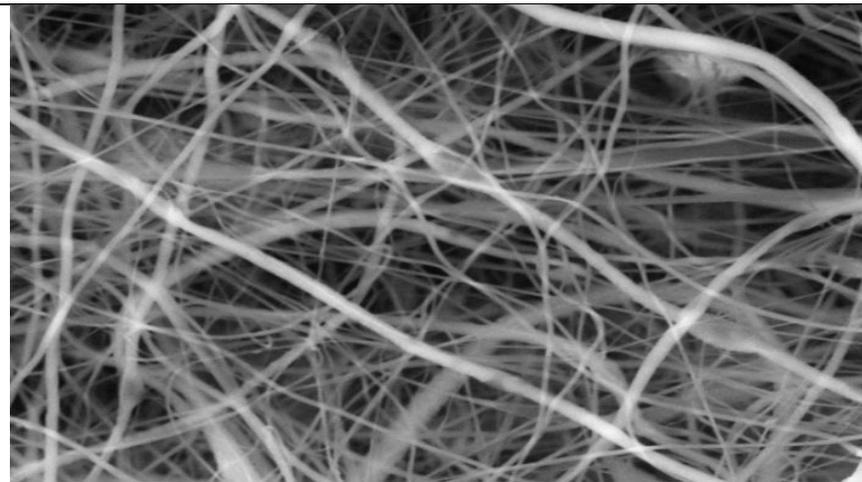
**Figure 4.12:**  $3.75 \times 10^{-4}$ M PCL 2 mixed with Titanocene Dichloride drug embedded nanofibers
