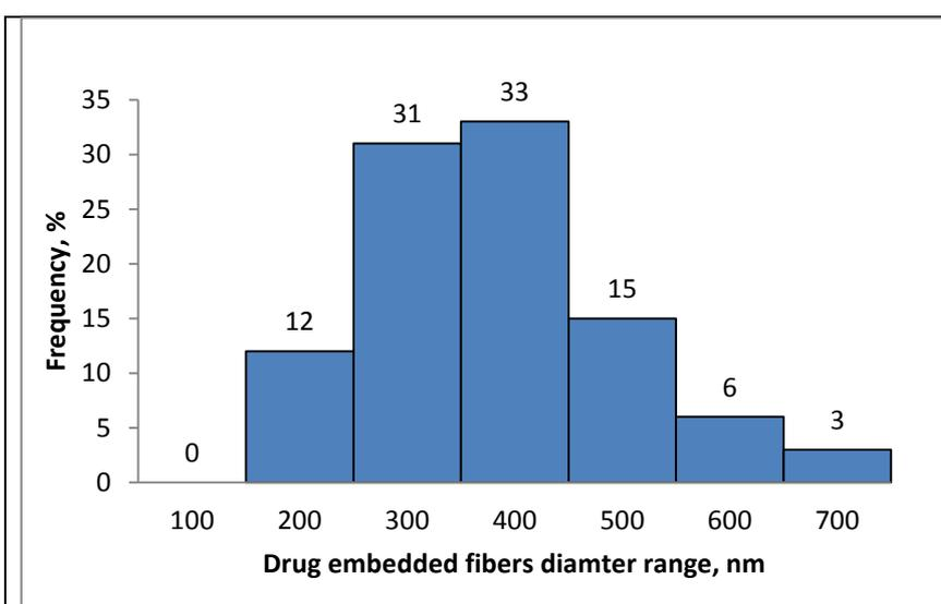
**Figure 4.14:** Fibers Diameter of Titanocene embedded Nanofibers
