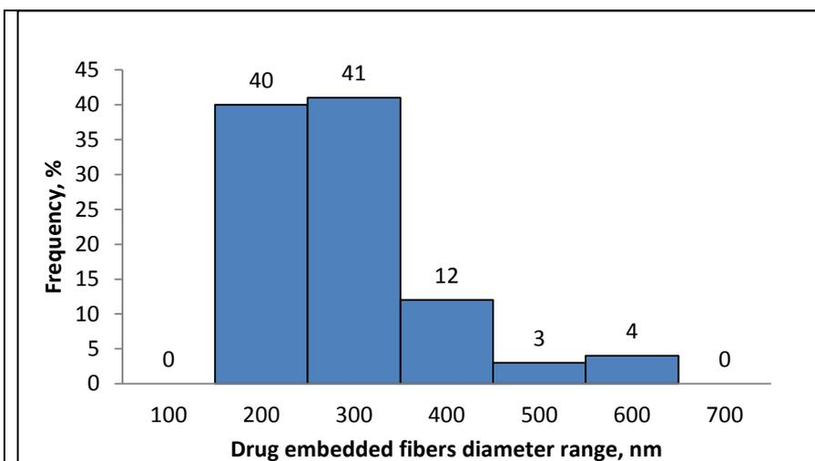
**Figure 4.13:** Fibers Diameter of Curcumin embedded Nanofibers
