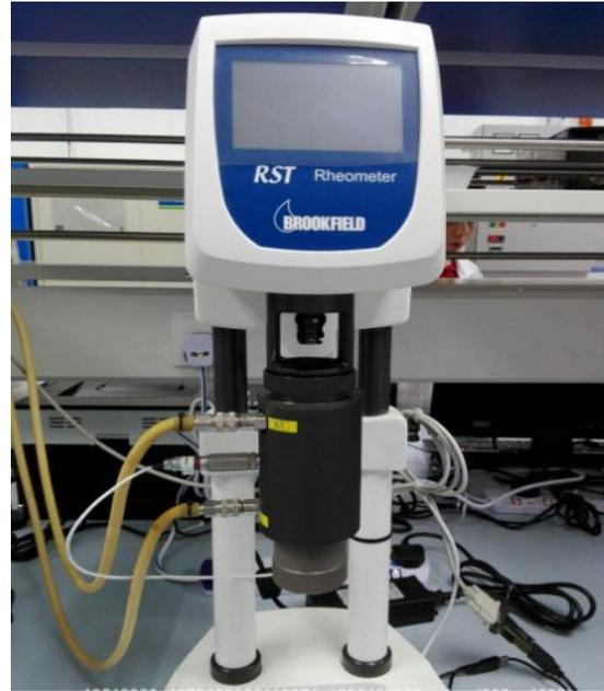
Figure 3.2: rheometer fitted with a CCT 25 coaxial spindles
