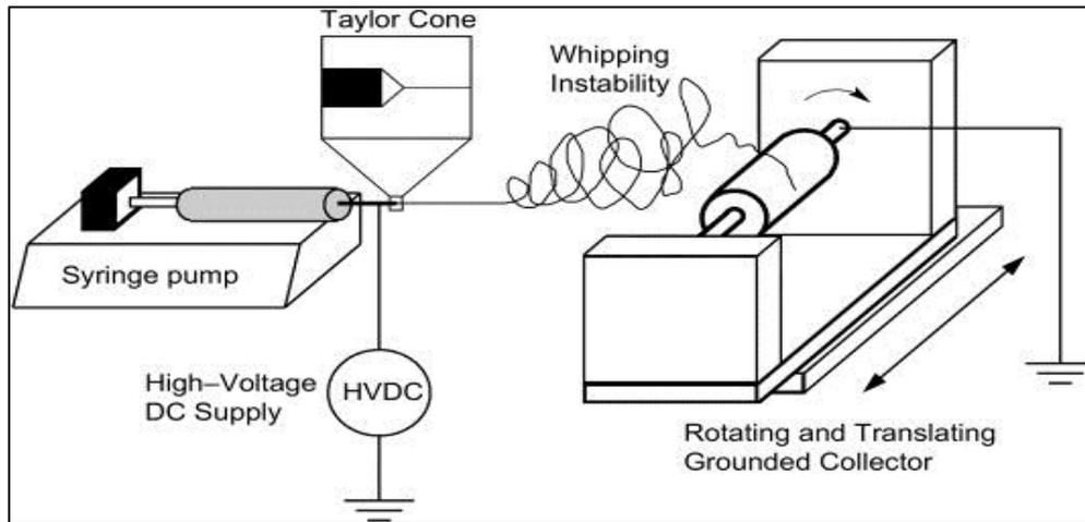
**Figure 0.1:** the schematic of typical electrospinning system (Wang et al., 2011)
