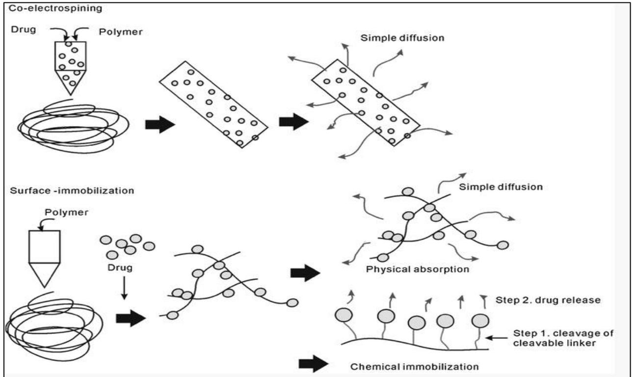
**Figure 0.3:** Schematic diagram of simple drug loading method within the nanofiber or on the surface of the nanofiber and its release kinetics. (Son et al., 2013)
