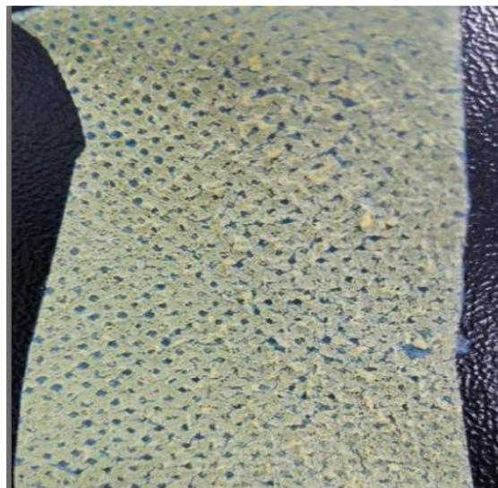
**Figure 4.16:** Surface of PEO mixed with ethanol and distilled water + titanocene dichloride
