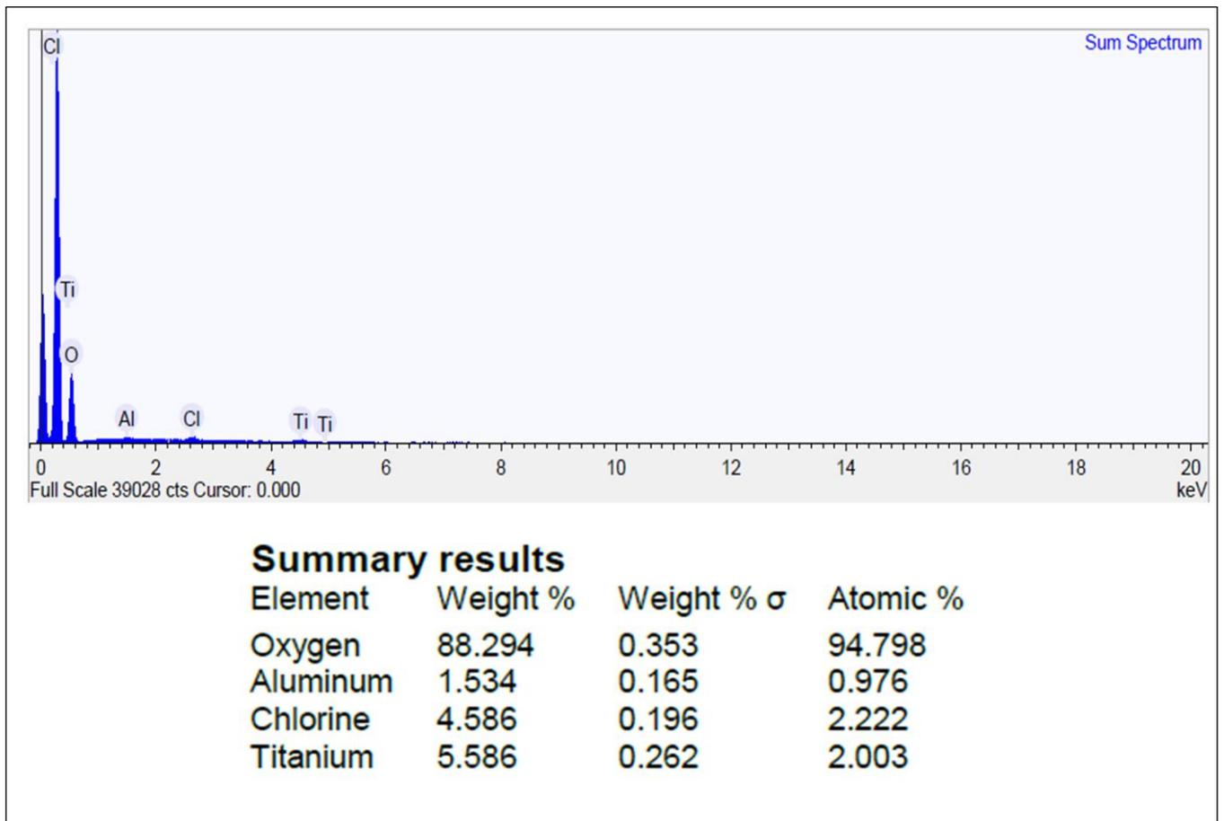
**Figure 4.19:** Composition of PCL embedded with titanocene dichloride measured by EDX
