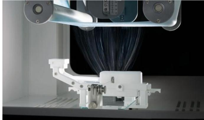
**Figure 0.2:** Needleless wire Electrospinning Process (Nanospider™) (Wang et al., 2011)
