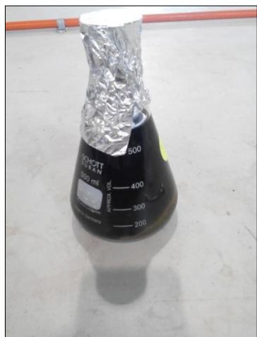
A1-8: Extraction of palm oil leaves powder by using methanol and stir by using magnetic stirrer and hotplate.
