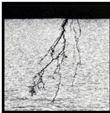
Figure 2.12 : Cross section of typical cracking corrosion
