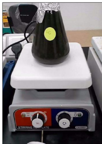
A1-8: Extraction of palm oil leaves powder by using methanol and stir by using magnetic stirrer and hotplate.
