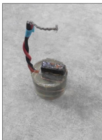
A1-7: The electrode obtained after mounded with epoxy solution
