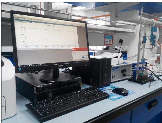
A1-10: Electrochemical measurement by using potentiostat as equipment, polarization resistances test were carried out.
