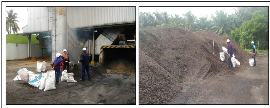
Figure 1: Unground POFA and oil palm shell packed in gunny at the dumping area of oil palm mill.
